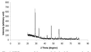
Fig. 4. XRD pattern of the xerogel obtained from complex 1 heated to 600  $^{\circ}\text{C}.$
