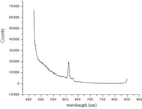
Fig. 6. Eu<sup>III</sup> photoluminescence spectrum (at 440 nm excitation wavelength) of the xerogel obtained from  $Gd(OPr^i)_3$  and heated to 900 °C.
