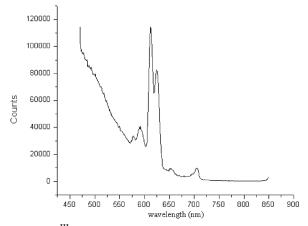
Fig. 5. Eu<sup>III</sup> photoluminescence spectrum (at 440 nm excitation wavelength) of the xerogel obtained from complex 1 which was heated to 600  $^{\circ}$ C.
