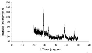
Fig. 3. XRD pattern of the xerogel obtained from  $Gd(OPr^{i})_{3}$  heated to 900 °C.
